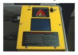
Calibrates electrofusion control boxes in the field and troubleshoots control box malfunctions.
